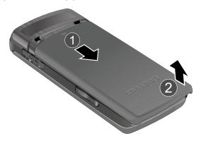
2. Lift the battery up (1) and away (2) from the phone, as shown.
