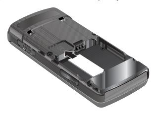
3. To remove the SIM, slide it gently out of the socket.
