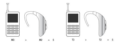
In the above example, if a hearing aid meets the M2 level rating and the wireless phone meets the M3 level rating, the sum of the two values equal M5. This is synonymous for T ratings. This should provide the hearing aid user with "normal usage" while using their hearing aid with the particular wireless phone. "Normal usage" in this context is defined as a signal quality that is acceptable for normal operation.
