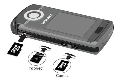
2. Push the microSD<sup>™</sup> card into the slot until it clicks into place.
