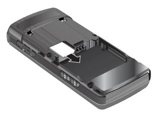
**Note:** The angled corner of the SIM should be inserted as shown above. The correct insertion is shown on the phone itself. Improperly inserting the SIM can cause the phone to not recognize the SIM.
