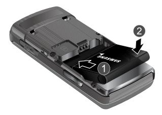
3. With the battery in position in the phone, align the tabs at the bottom of the battery cover with the slots on the handset (1) and slide the cover down (2) until it clicks.
