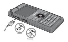
Note: The previous illustration shows both the correct and incorrect method for connecting the charger. If the incorrect method is attempted, damage to the accessory port will occur therefore voiding the phone's warranty.
