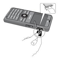
To remove the card, a quick press releases the card from the slot.
