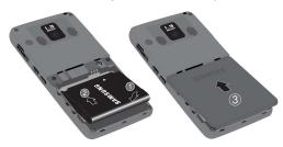
With the battery in position on the phone, place the cover back on the handset and slide it in until it clicks.
