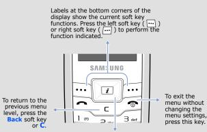
Use the 4-way navigation keys to scroll up, down, left, or right through the menu system, highlight menu items, and change feature settings
