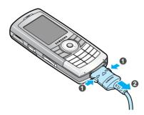
**Note**: Do not remove the battery while the phone is connected to an AC wall outlet. It may cause malfunctions and may damage the phone.
