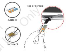
Note: If the card is not inserted correctly, the device will not detect the SIM card. Re-orient the card back into the slot if the SIM is not detected.
