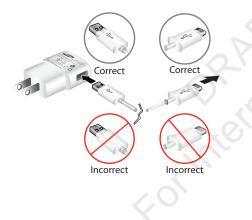
Insert the USB cable into the device's Charger/ Accessory Port (2).
