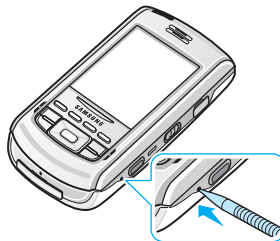
RESET key inside the hole
