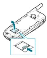
4. Insert the SIM card, ensuring that the cut corner faces top left and the gold contacts of the card face into the phone
