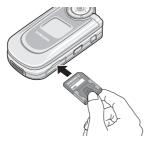
To remove the memory stick, press and release the card so that it is disengaged from the slot. Then slide it out.
