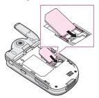
**Note:** When you need to remove the SIM card, slide it upwards, as shown, and take it out of the socket.
