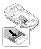
Note: When you need to remove the SIM card, slide it, as shown, and take it out of the socket.
