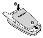
Press the battery down until it clicks into place. Make sure that the battery is properly installed before switching on the phone.
