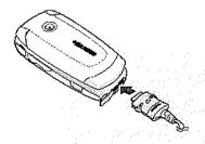
Plug the adapter into a standard AC wall outlet.
