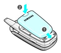
**6.** Press the battery down until it clicks into place. Make sure that the battery is properly installed before switching on the power.
