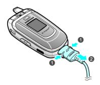
**Note:** You must unplug the charger before removing the battery from the phone during charging, otherwise, the phone could be damaged.
