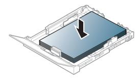
For paper smaller than Letter-sized, press and unlatch the guide lock in the tray, push the tray in manually. Then adjust the paper length guide and paper width guide.
