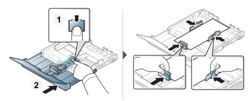
For paper longer than A4-sized(like 'Legal'), press and unlatch the guide lock in the tray, pull the tray out manually. Then adjust the paper length guide and paper width guide.
