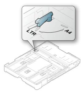
3 Squeeze the paper width guide and slide it to the edge of the lever.
