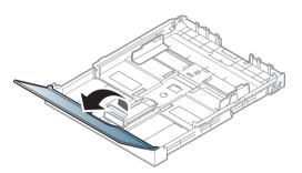
Press and unlatch the guide lock in the tray, pull the tray out manually. Then adjust the paper length guide and paper width guide.
