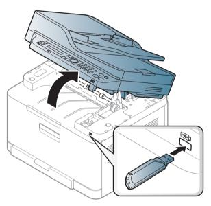
The USB memory port on the front of your machine is designed for USB V1.1 and USB V2.0 memory devices. Your machine supports USB memory devices with FAT16/FAT32 and a sector size of 512 bytes.
