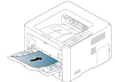
3 Squeeze the Multi-purpose (or Manual feeder) tray paper width guides and adjust them to the width of the paper. Do not force them too much, or the paper will bent resulting in a paper jam or skew.
