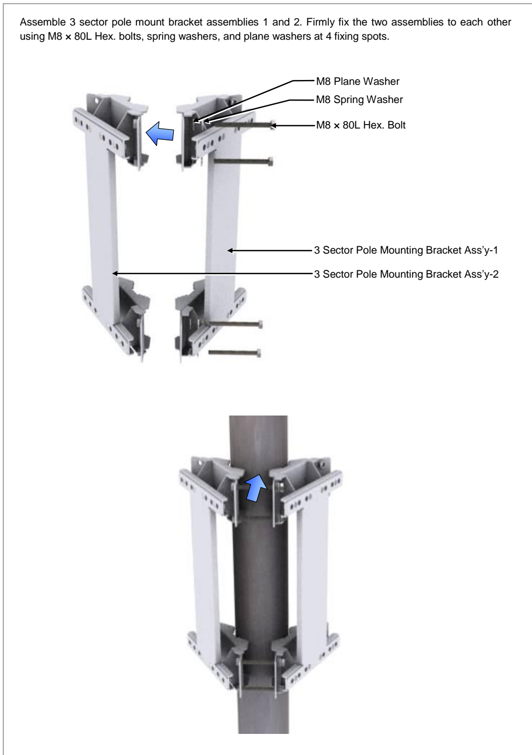
Figure 2.15 Fixing 3 Sector Pole Type RRH-2WB (2)
