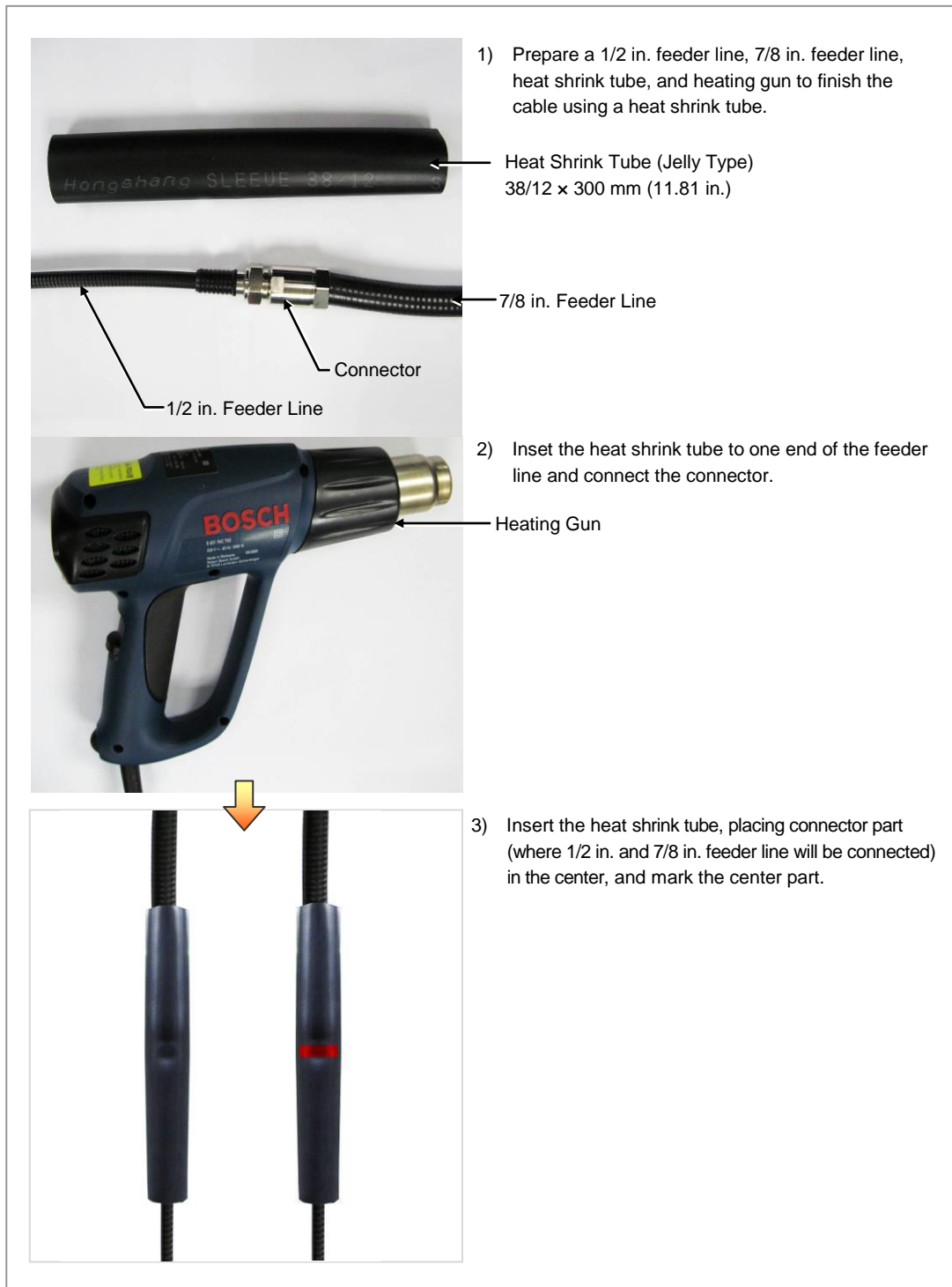
Figure C.10 Shrinking the Heat Shrink Tube_Connection between Connectors (1)
