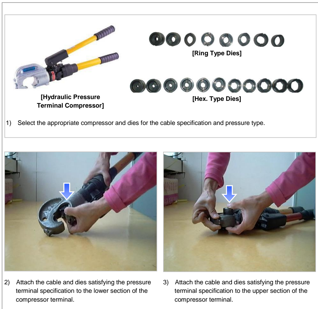
Figure E.1 Pressure Terminal Assembly (1)
