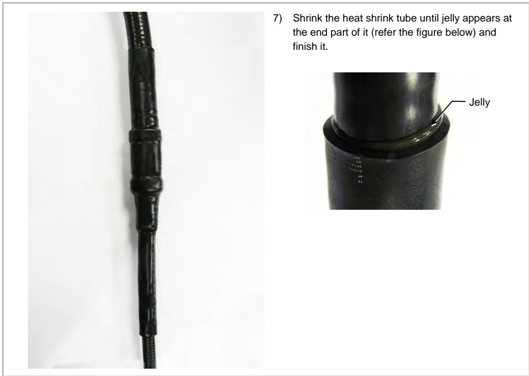
Figure C.12 Shrinking the Heat Shrink Tube_Connection between Connectors (3)
