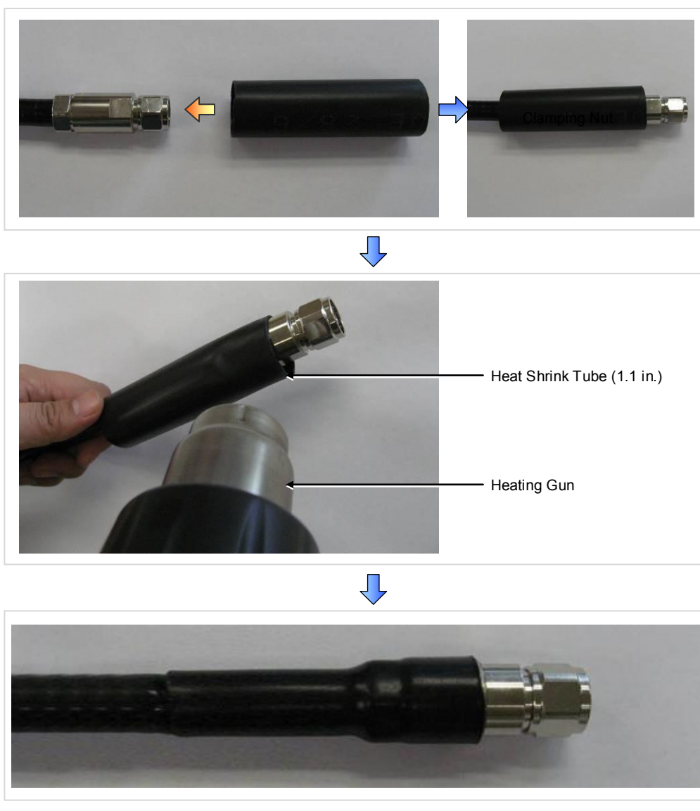
Figure C.11 Assembling the N type-male (1/2 in. Feeder Line) Connector (4)
