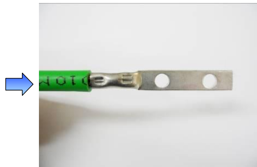
Figure F.7 Fixing Pressure Terminal_Handheld Compressor (2)
