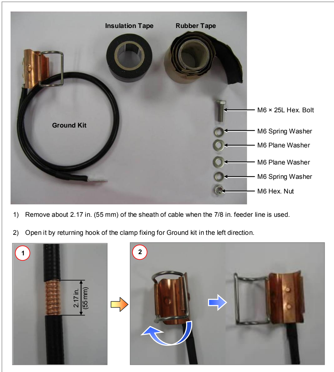
Figure B.1 7/8 in. Feeder Line Grounding (1)
