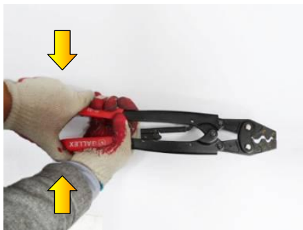
Figure F.7 Fixing Pressure Terminal_Handheld Compressor (2)
