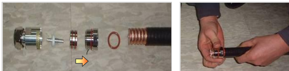
Figure C.12 Assembling the Din type-male (1/2 in. Feeder Line) Connector (1)
