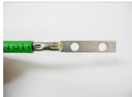
Figure E.7 Fixing Pressure Terminal_Handheld Compressor (2)
