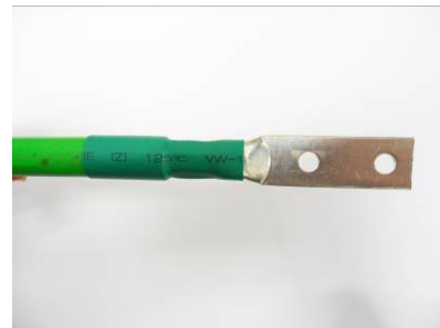
Figure E.10 Assembling Heat Shrink Tube
