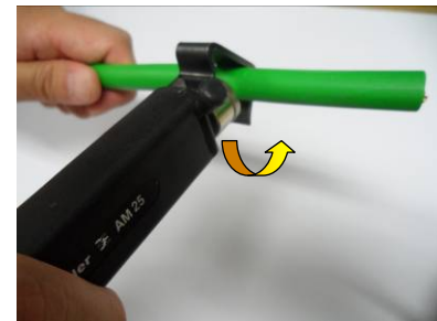
Figure E.4 Stripping Cable Sheath (1)
