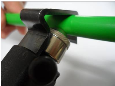
Figure E.4 Stripping Cable Sheath (1)
