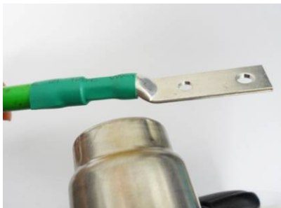
Figure E.10 Assembling Heat Shrink Tube
