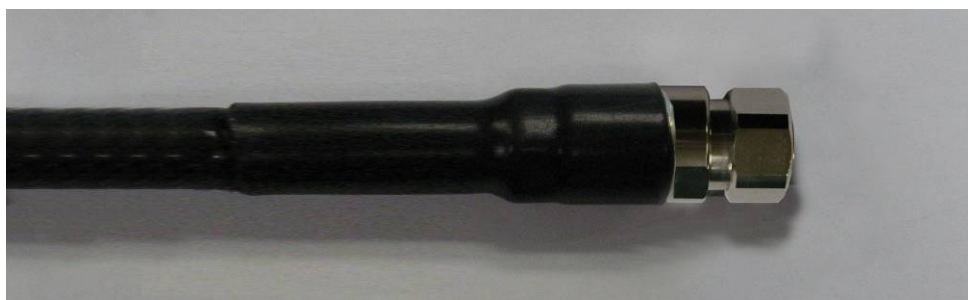
Figure C.13 Assembling the Din type-male Connector (1/2 in. Feeder Line) (2)
