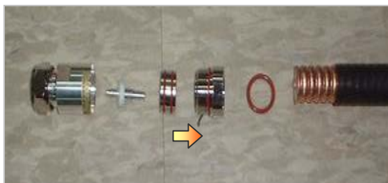
Figure C.12 Assembling the Din type-male Connector (1/2 in. Feeder Line) (1)
