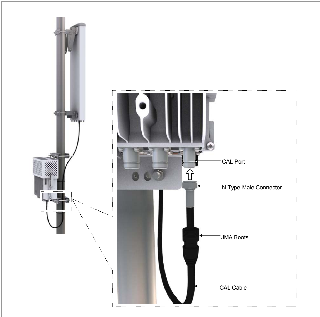
Figure 27. Connecting CAL Cable_Type 1 (1)
