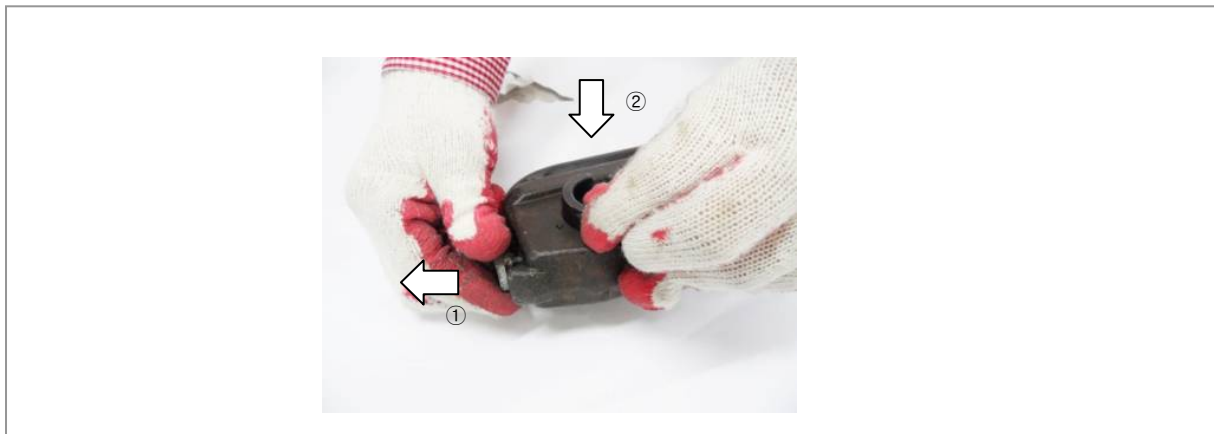
Figure 96. Fixing Pressure Terminal_Hydraulic Press (2)
