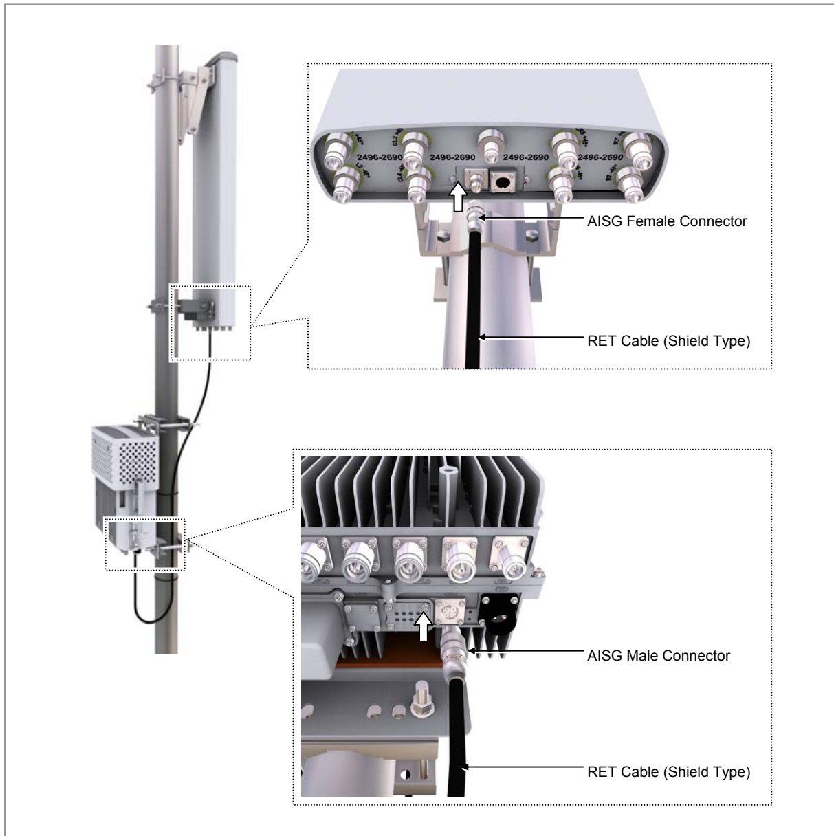
Figure 25. Connecting RET cable
