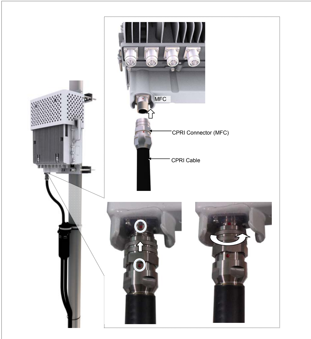
Figure 65. Connecting CPRI Cable_Type 1 (15)
