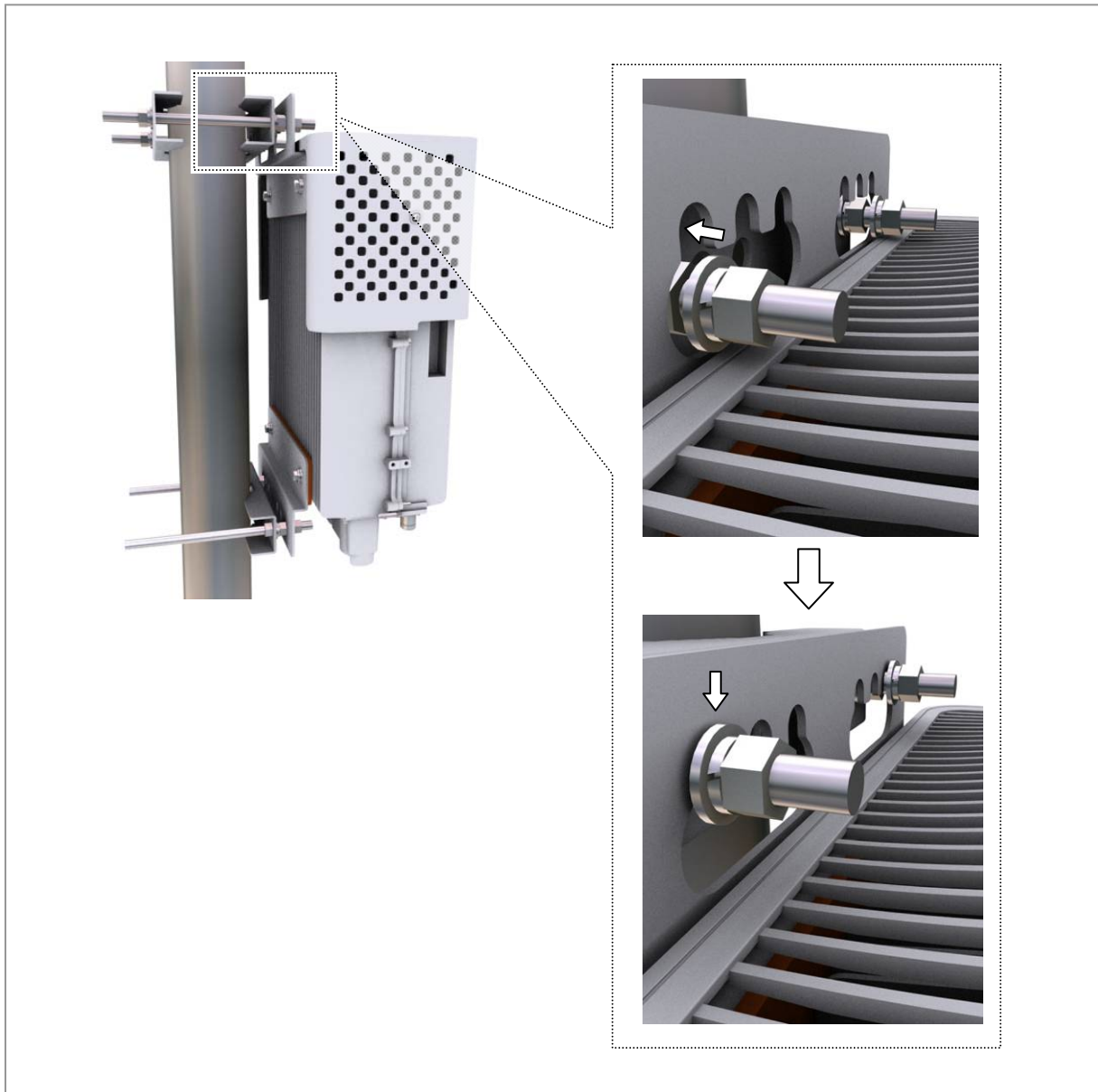
Figure 16. 1 Sector Pole Fixation (6)
