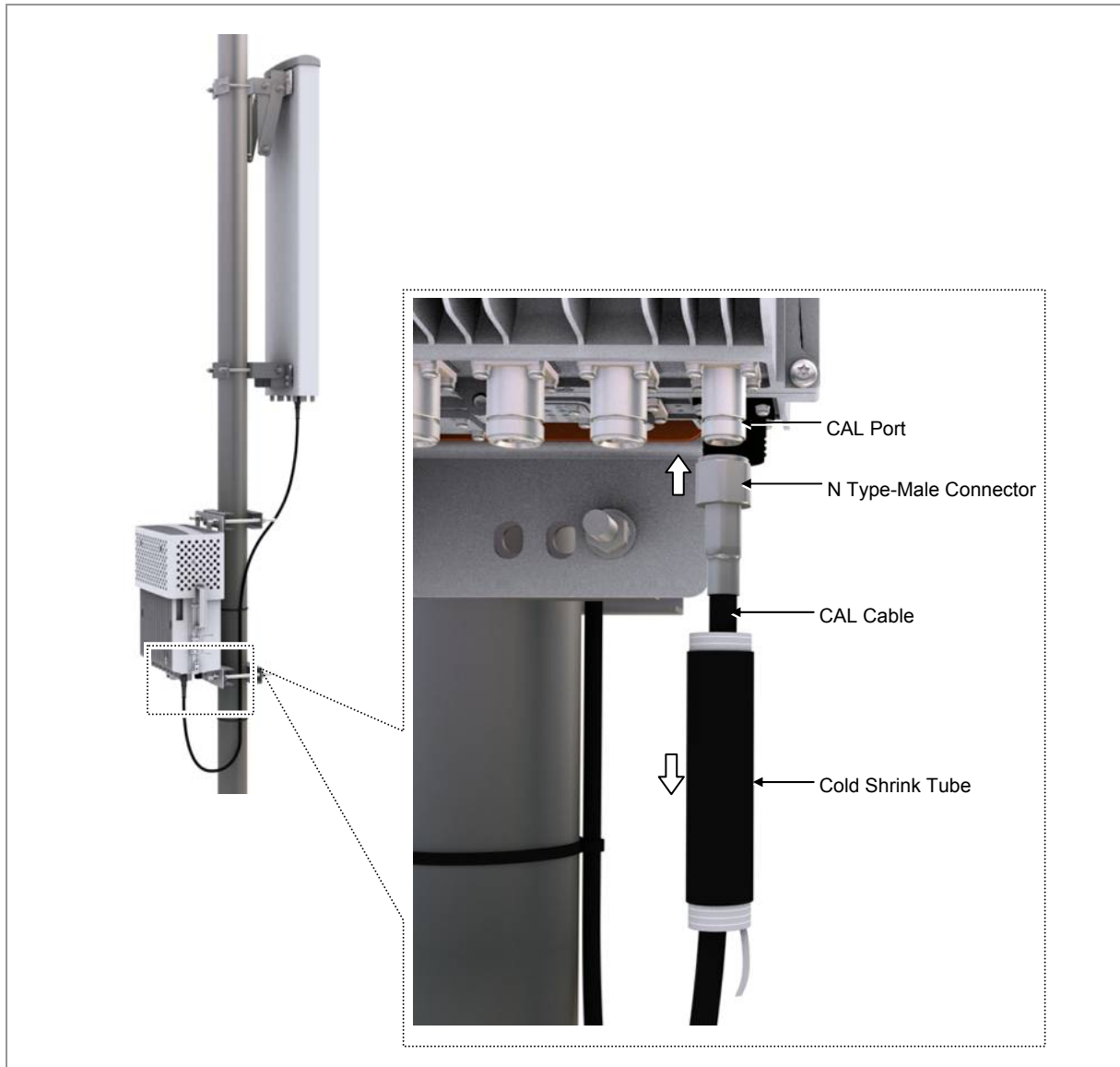
Figure 30. Connecting CAL Cable_Type 2 (1)
