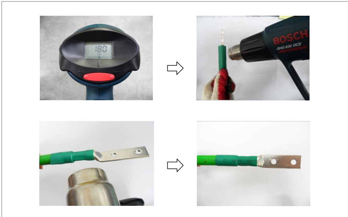
Figure 101. Assembling Heat Shrink Tube (2)
