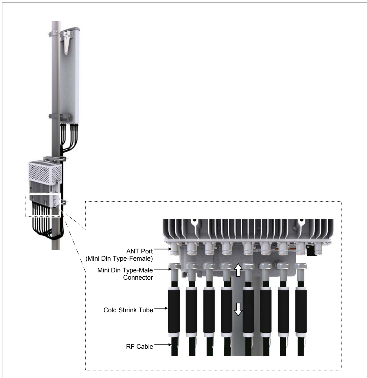
Figure 22. Connecting RF Cable_Type 2 (1)
