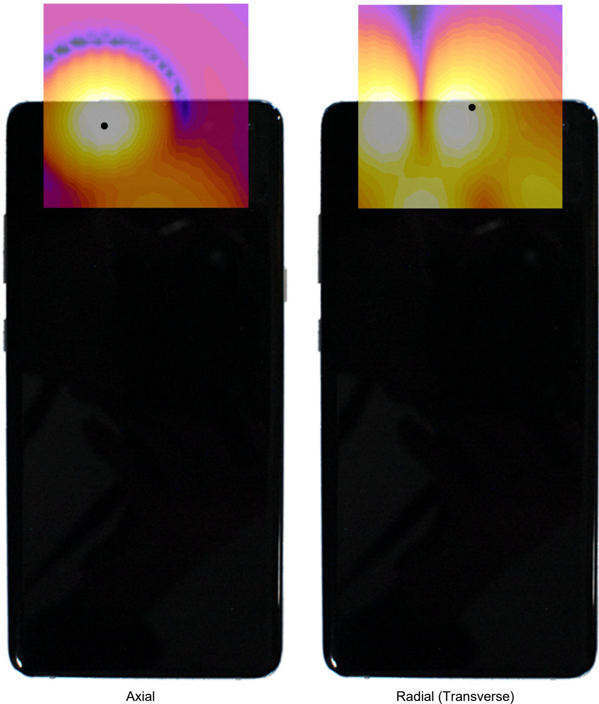
Figure 16-3 T-Coil Scan Overlay Magnetic Field Distributions
