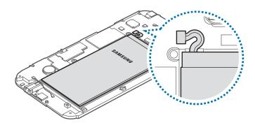
6 Push the back of the battery with your fingers and remove the battery.
