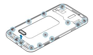
4 Remove the circuit board by lifting it out of the case using an opening tool, then put the case aside and place the circuit board face down on a flat work surface.
