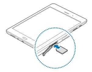
3 Push the SIM or USIM card into the slot until it locks in place.
