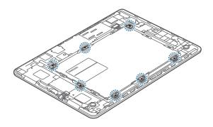
5 Disconnect the battery connectors as shown in the image below.
