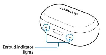
Colour **Status** Continuously on red • Charging Continuously on green • Fully charged Flashes red (rapid pace) • Charging disabled due to abnormal temperatures Charging disabled due to an error in connecting to the charging contacts Flashes red (medium pace) Charging disabled due to low charging case battery ٠
