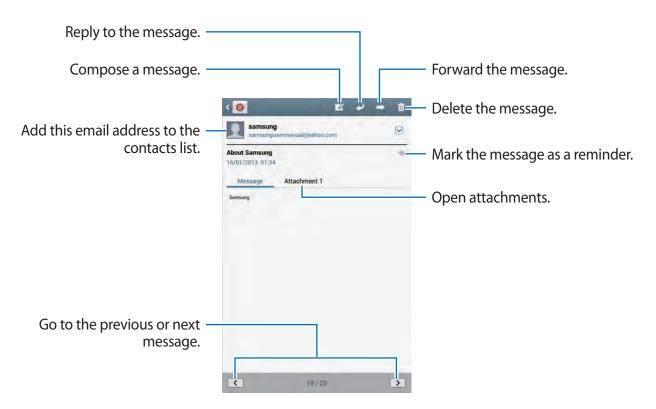
Tap the attachment tab to open attachments, and then tap **Save** next to an attachment to save it.
