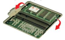
**b.** Hold the memory module by the edges and pull it forward out of the compartment.
