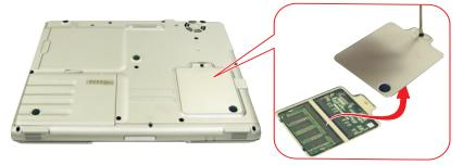
3. Grasp the edge of the door and pull the door off the chassis.
