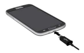
3. Plug the other end of the USB cable into the Charging Head, and then plug the Charging Head into an electrical outlet to charge your battery. Fully charging a battery may take up to three hours.
