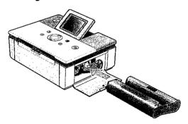
**6** Make sure that the cartridge is under the lever and then close the side cover.
