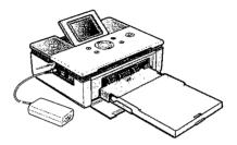
2 Connect the power cord to the power adapter and connect the cord to the wall outlet or power source.
