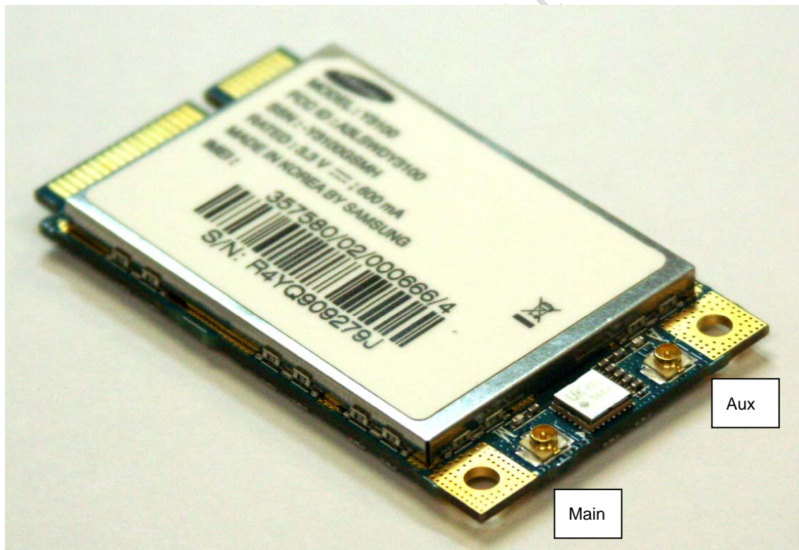
Figure 8. placement of the antenna connectors for Y3100
