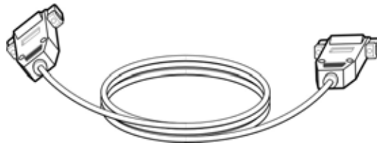
Figure 5.17 Connecting Cable of the Console Terminal
