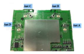
Inverted F-type antennas are used for both wireless modules and four antennas are used for receive mode, two antennas are used for transmission mode.
