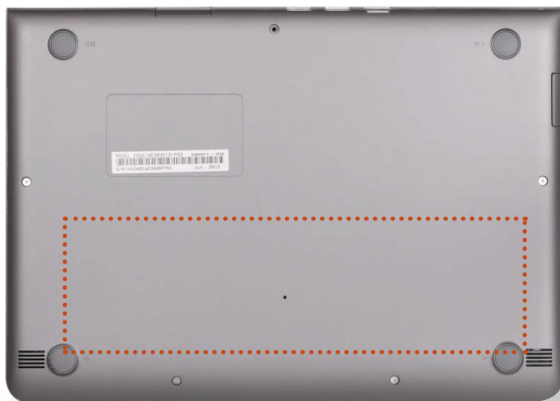
The location of the internal battery
