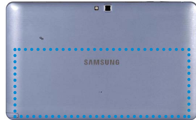
The location of the internal battery
