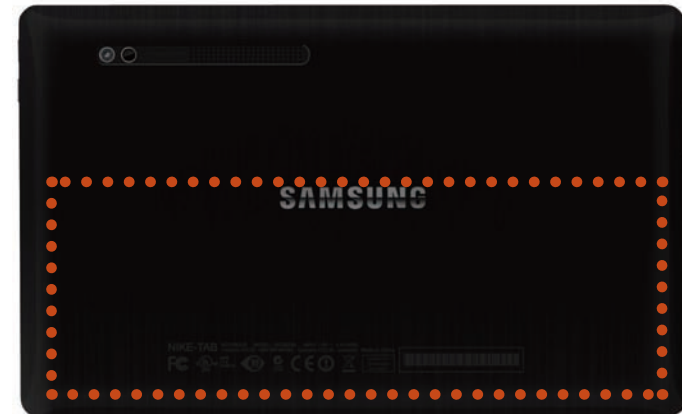
The location of the internal battery
