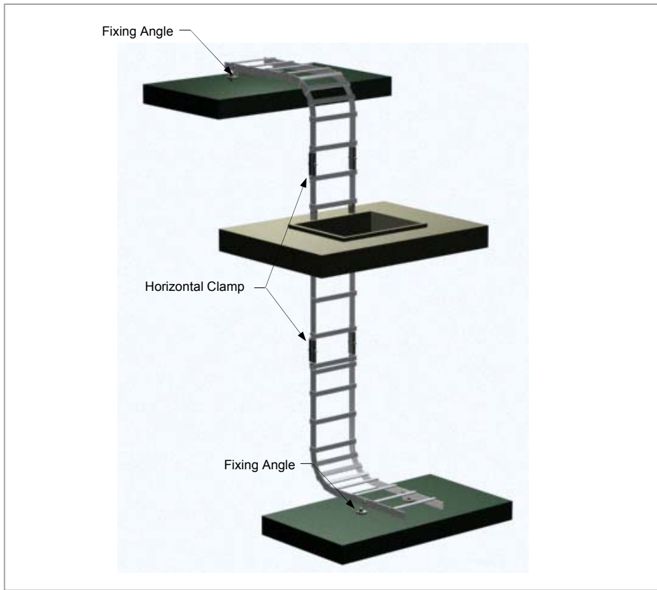
Figure 2.12 Installing Upper/Lower Curved Cable Rack
