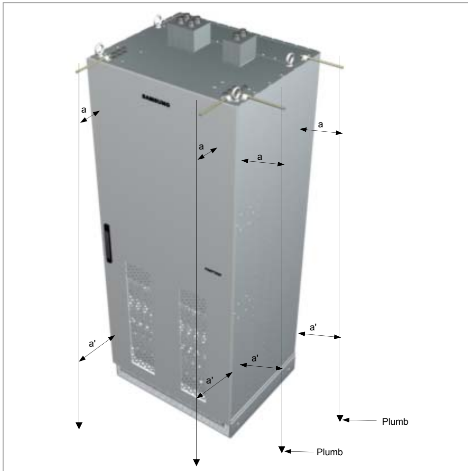
Figure 2.31 Leveling by a Plumb
