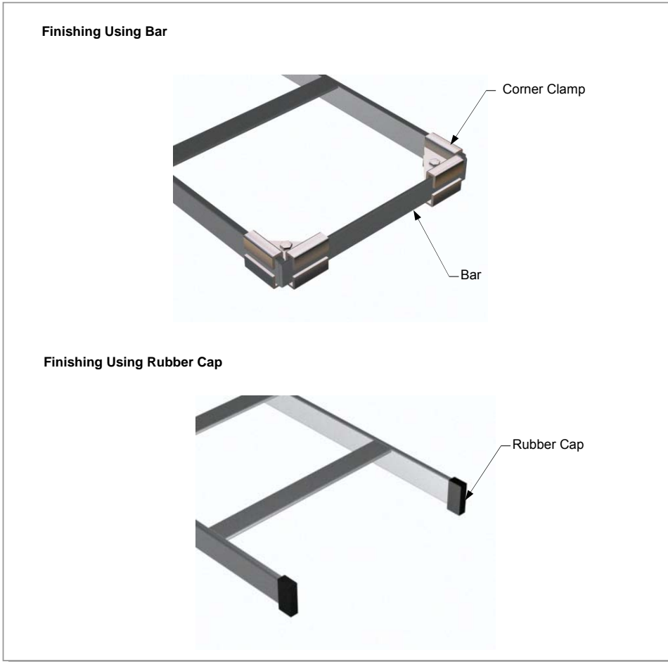
Figure 2.18 Cable Rack Finishing
