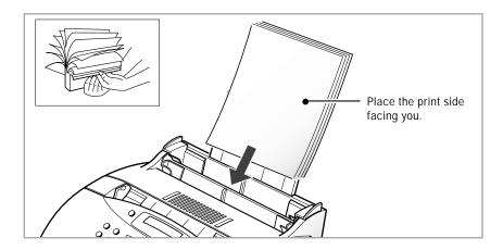
• Load letterhead paper with the design facing you. The top edge of the sheet with the logo should enter the printer first.
