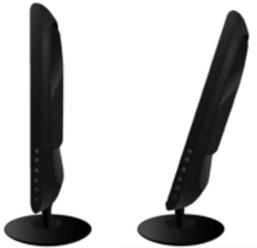
You can adjust the tilt angle within a range of 0° forward to 20° backward for the most comfortable viewing angle.
