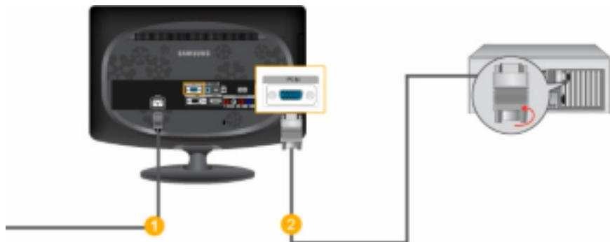
1 Connect the power cord for your monitor to the POWER port on the back of the monitor.
