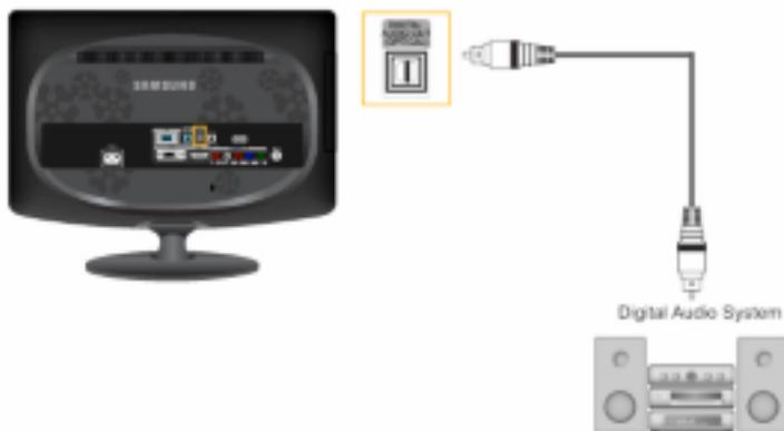
1. Connect the *[DIGITAL AUDIO OUT (OPTICAL)]* terminal of your monitor to the digital sound input terminal of your digital amplifier using an optical cable.
