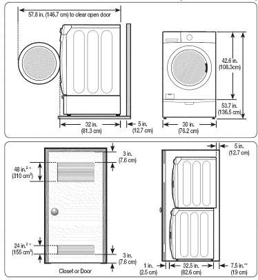
Required Dimensions for Installation With Stacking Kit (Model No.: SKK-BB)
