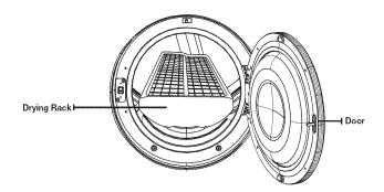
Place the Drying Rack inside the dryer, align the holes of the filter handle of the Drying Rack with the front projections, and then secure the back of the Drying Rack.
