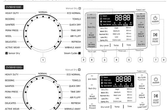
To select a cycle, rotate the Cycle Selector dial to the desired cycle. The indicator light by the cycle name will illuminate. The NORMAL, HEAVY DUTY, BEDDING, SANITIZE, PERM PRESS, WOOL, DELICATES, ACTIVE WEAR, ECO NORMAL, and TOWELS cycles are Sensor Dry cycles. Sensor Dry automatically senses the moisture in the load and shuts the dryer off when the load reaches the dryness level you have selected with the Dry Level Selection Button (see below).
