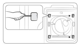
**5.** Use a flat-head screwdriver to remove the two hinge covers from the original side. Install the hinge covers on the opposite side as shown.
