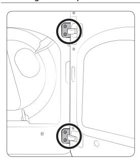
To reverse the direction of the door, we recommend that you contact a qualified technician. It is recommended to put a soft rug on the floor to prevent scratches on the door.
