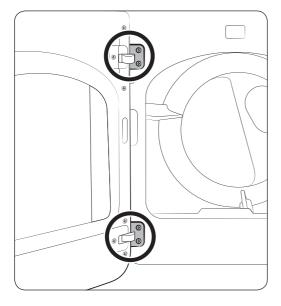
**11.**Reinstall the door on the front frame, and then carefully insert and tighten the 4 hinge screws.
