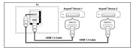
Connect the [HDMI 1] or [HDMI 2] jack on the TV and the HDMI OUT jack of the corresponding Anynet<sup>+</sup> device using an HDMI cable.
