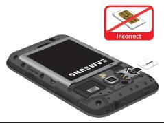
Note: If the SIM card is not inserted correctly, the phone cannot make an LTE connection with the network.
