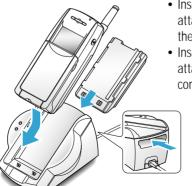
Insert the entire phone with battery attached into the front compartment of the charger.
