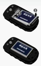
4. With the battery in position on the phone, place the cover back on the handset and use the battery cover removal tool to turn the grooved dial clockwise until the cover locks.
