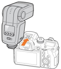
3 Rotate the hot-shoe fastening dial as shown in the illustration to lock the flash into place.
