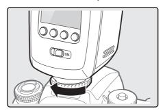
4 Slide the power switch towards **ON** to turn on the flash.
