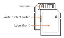
You can prevent files from being deleted by using the write-protect switch on an SD, SDHC, or SDXC card. Slide the switch down to lock or slide it up to unlock. Unlock the card when capturing photos and videos.
