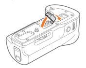
Align the electrical contacts, the mounting screw, and the camera guide pin with the bottom of the camera.
