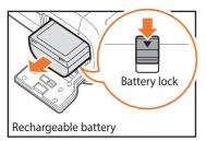
Slide the lock down to release the battery.
