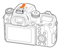
Mount the flash by sliding it into the hot-shoe.
