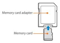
To use micro memory cards with this product, a PC, or a memory card reader, insert the card into an adapter.
