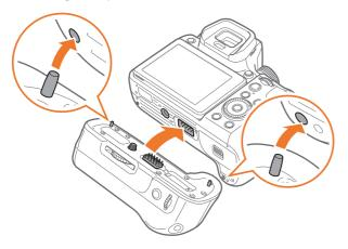
3 Lock the vertical grip in place by turning the vertical grip locking dial to LOCK.
