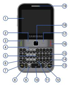
Display: Shows information needed to operate your phone: signal strength, battery level, time and date, and more.
