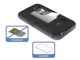
Make sure that the card's gold contacts face into the device and that the upper-left angled corner of the card is positioned as shown.
