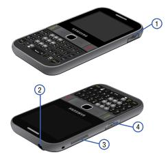
USB Power/Accessory connector: Allows you to connect a power cable or optional accessories such as a USB/ data cable.
