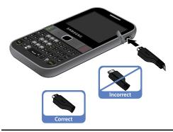
Important! Verify that the handset battery is installed prior to connection. If the battery is not properly installed and the wall charger is connected, the handset may power off and on continuously, preventing proper operation.
