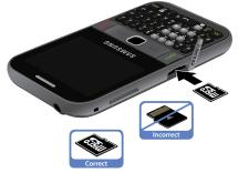
**3.** Once secured, put the cover back into place to cover the opening.
