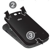
**Caution!** Do not bend or twist the back cover excessively. Doing so may damage the cover.
