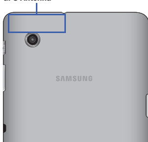
Location of Internal GPS Antenna
