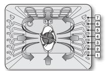
By using the convection bake feature, you will be able to cook faster. You can program the oven for convection baking at any temperature between 150°F and 550°F.
